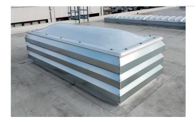
Easy-to-install base for continuous ventilation, designed in detail using 3D modeling. It comprises Z-shaped moulded fins that are fitted to the structural element and installed on a waterproofed curb. The dimensions and finishes can be customized to suit individual requirements.
